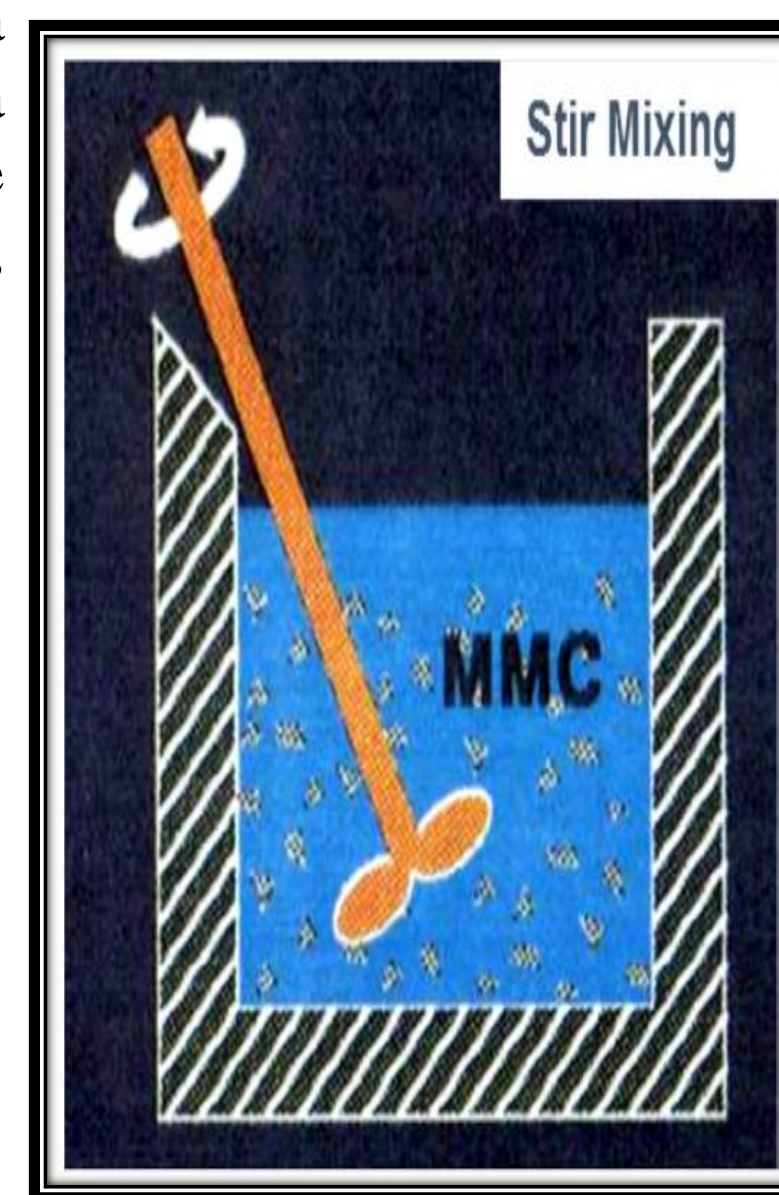
Figure 10 Schematic Representation of Stir Casting
