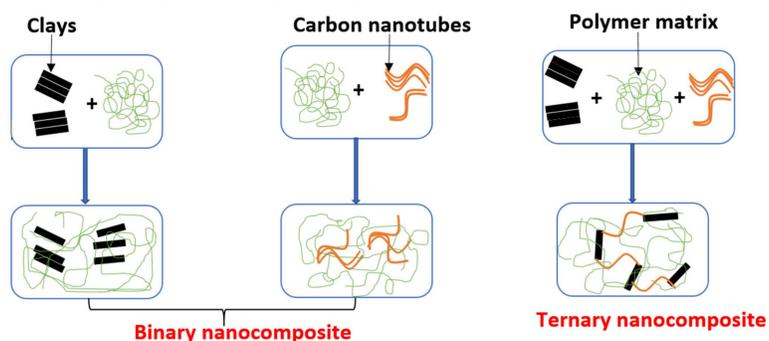
Using MMT to disperse CNT, reduce percolation threshold and create 3D network structure of nanofillers [1]
