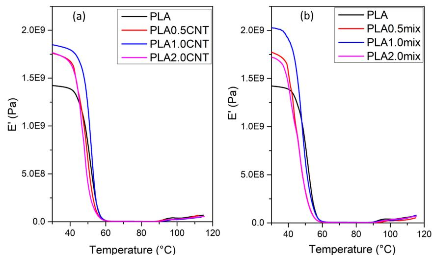
Addition of MMT & CNT resulted in the optimum storage modulus ( $E'$ ) of 2.03 GPa in PLA1.0mix, compared with PLA/CNT
