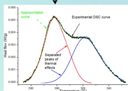
Fig. 3. Peak separation from overlapping effects by Gaussian distribution
