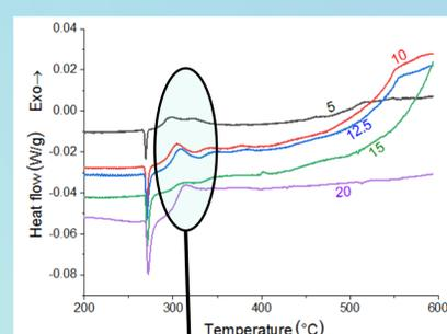
Fig. 2. DSC scans for  $\text{Sn}_{0.9}\text{Pb}_{0.1}\text{Te}$  with different heating rates
