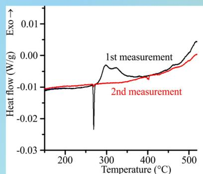
Fig. 1. Multiple DSC scans for  $\text{Sn}_{0.9}\text{Pb}_{0.1}\text{Te}$
