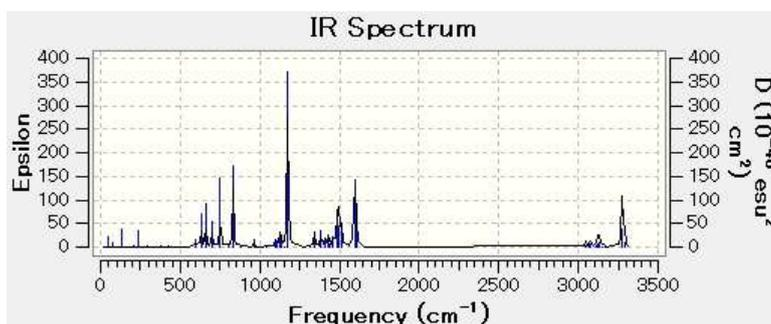
Fig 2. IR Spectrum of EMIm cation obtained by DFT.
