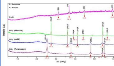
Fig. 6. XRD analysis of the products of thermal decomposition of TiL<sub>2</sub> and CoL<sub>2</sub>.2H<sub>2</sub>O.
