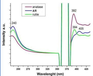
Fig. 8. Excitation spectra TiO<sub>2</sub> nanoparticles obtained at 370 nm with the use of Xe lamp.
