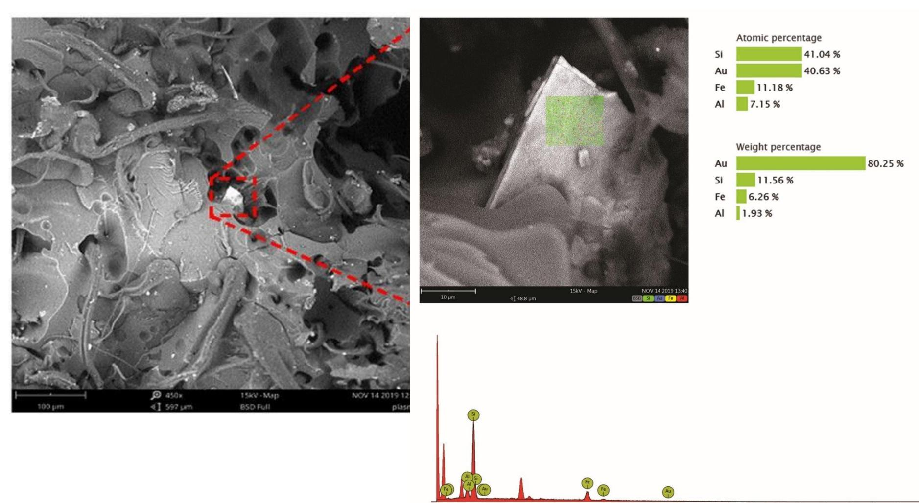
From the analysis, a substantial heterogeneity of the material clearly emerges, especially as regards the presence of non-polymeric particles. the presence of Silicon and Gold with an atomic concentration of 41.04% and 40.63% respectively. Less representative, aluminum and ferrous components (7.5% and 11.18%). It is conceivable that among the components of Plasmix there is plastic material used for the construction of electronic circuits.
